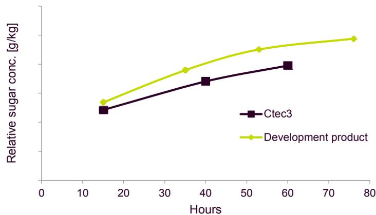
*Hydrolysis performance of the new enzyme cocktail and benchmark enzyme in the pilot plant*
