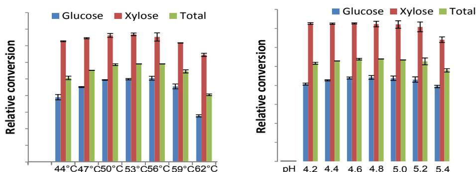
*Temperature and pH profiles evaluated in hydrolysis of pretreated substrate from Biochemtex pilot plant.*
